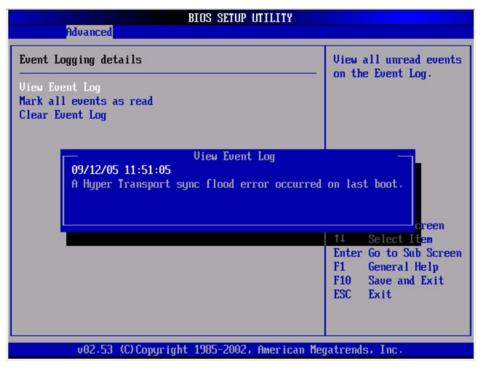
FIGURE E-1 Sample DMI Log Screen, Uncorrectable Error
