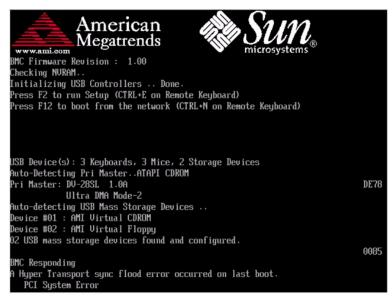
FIGURE E-5 Sample POST Screen, Previous System Error Listed
