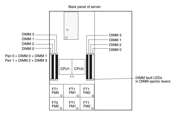
FIGURE 1-4 Sun Fire X4100/X4200 DIMM Slot Locations
