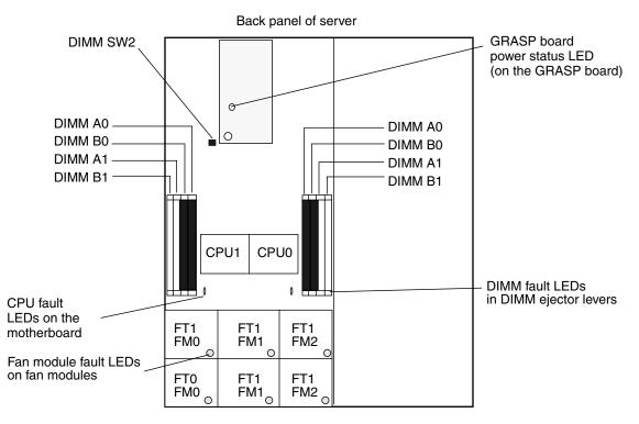
FIGURE B-4 Sun Fire X4100 M2/X4200 M2 Internal LED Locations
