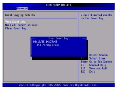
FIGURE E-4 Sample DMI Log Screen, PCI Parity Error
