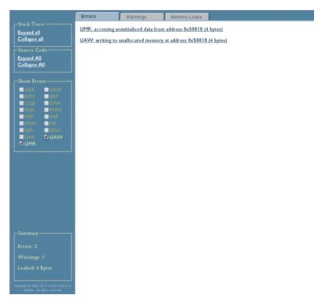
When you click on an error, the stack trace at the time of the error is displayed:
