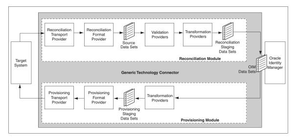
Figure 5–2 Functional Architecture of a Generic Technology Connector
