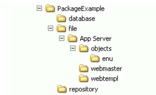
Figure 7. Example of ADM package directory structure created with the ADM Package Utility
