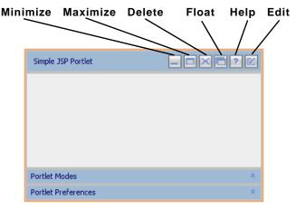
Figure 5-28 Portlet Mode and State Buttons in a Running Portlet
