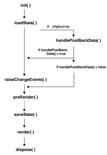
Figure 6-3 Flow of Portal Life Cycle Methods
