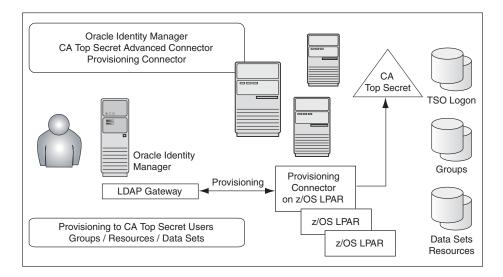
The Provisioning Connector includes LDAP bind and authorization requests. In addition to traditional provisioning functions, the Provisioning Connector can also build the necessary TSO logon functions, including the building CLIST files, and working to replicate existing mainframe user profile scenarios. Provisioning Connector can also extend authorization to data sets, groups, and resources through enterprise rules set in by Oracle Identity Manager.
