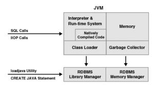
Figure 1–9 Main Components of the OracleJVM
