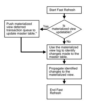
Figure 3-14 Fast Refresh of a Materialized View
