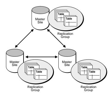
Figure 1-1 Multimaster Replication
