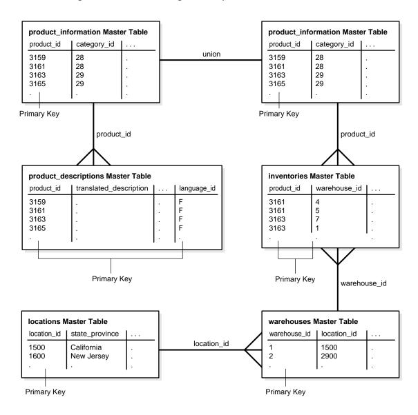
Figure 3–6 Row Subsetting with Subqueries and Unions
