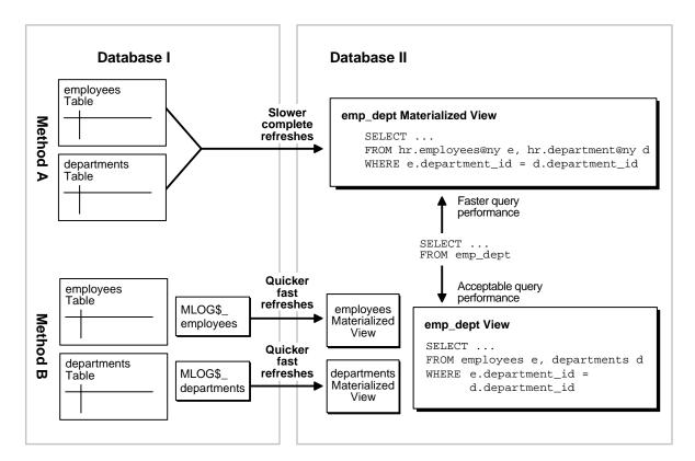
Figure 3–2 Comparison of Simple and Complex Materialized Views
