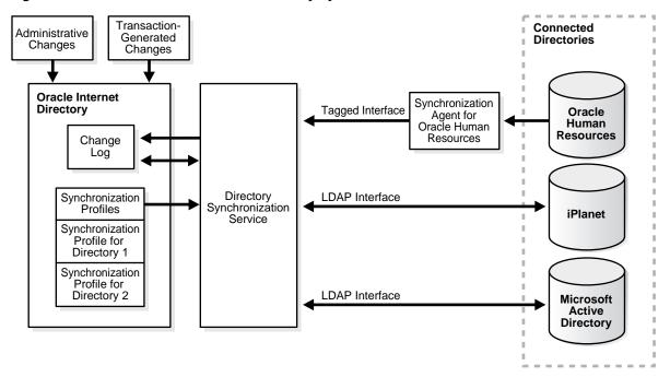
Figure 27–2 Interactions of the Oracle Directory Synchronization Service
