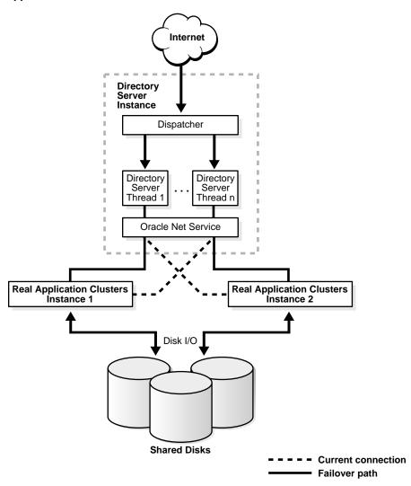
Figure 25–2 Single Directory Server Instance on One Node and Multiple Real Application Clusters Instances
