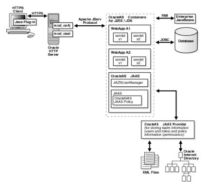
Figure 6–2 Oracle Component Integration In SSL-Enabled J2EE Environments
