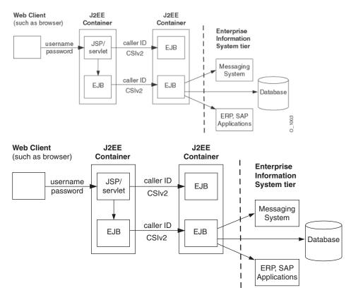
Figure 1–1 Identity Propagation Using CSIv2
