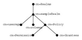
In an identity management-based environment, a subscriber is registered as a realm. Using the subscriber DN, the JAAS Provider locates the subscriber-specific Oracle Context and creates a cn=JAZNContext subtree. In this case, the JAAS Provider stores the entries cn=usermgr and cn=rolemgr and policy-related entries under the subscriber's JAZNContext.
