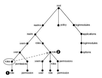
In this structure, the user and role nodes are linked together. This means that the roles link under user is the same link as the roles link under realm. In Unix terms, the role at numeral 1 in the diagram is a symbolic link to role at numeral 2 in the diagram.
