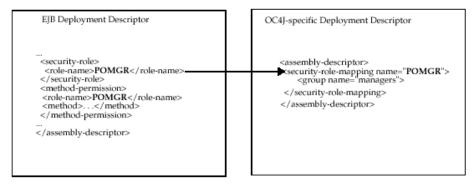
Notice that the <role-name> in the EJB deployment descriptor is the same as the name attribute in the <security-role-mapping> element in the OC4J-specific deployment descriptor. This is what identifies the mapping.
