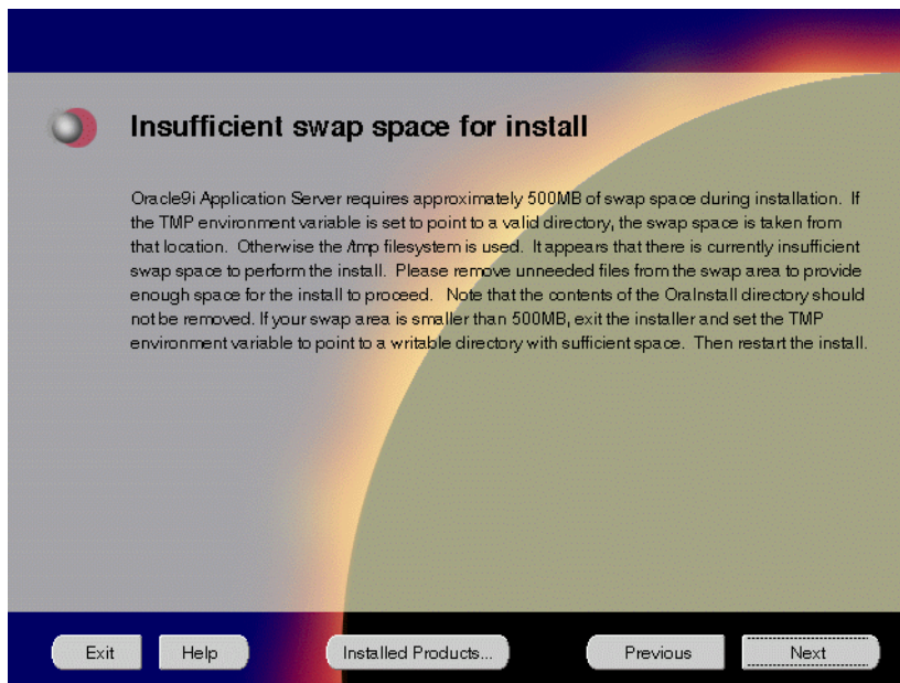
Figure 6–6 Insufficient Space in TMP Screen
