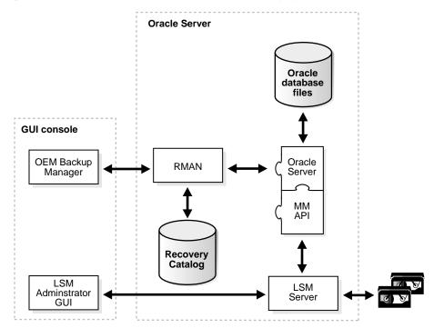
Figure 1–2 Oracle8 or Oracle8i Backup and Recovery System
