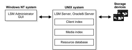
Figure 1–1 LSM Components
